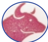
Medium PE tape print quality after 1 hour and 45 minutes, with no adjustments.
